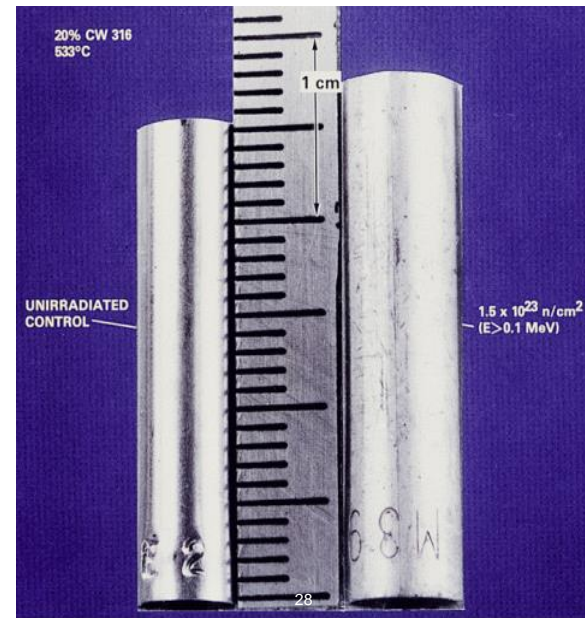
Radiation swelling of 316 stainless steel [4]
